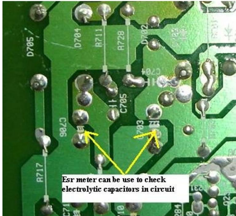
There are two different ways to test capacitors, one for the electrolytic capacitor and the other one for the non-polar or the ceramic type capacitor that do not have polarity. I will start explaining the electrolytic capacitor first. I believe many of you already own the ESR meter for testing electrolytic capacitor on board.
