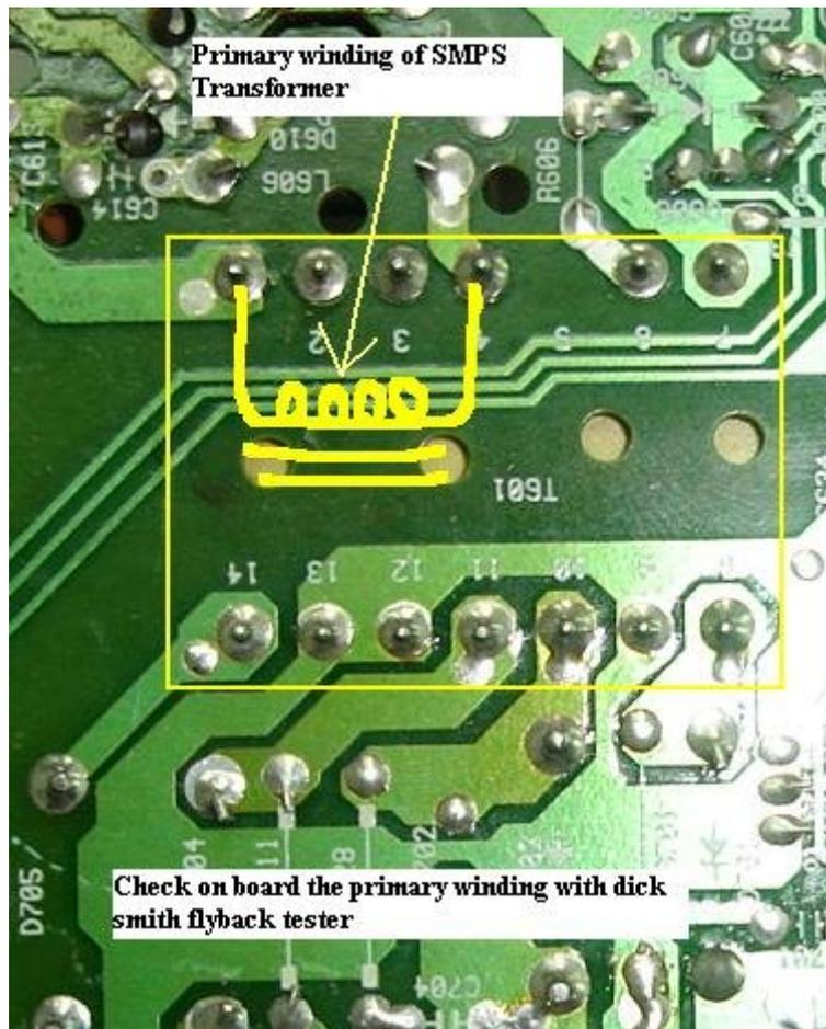
As for the switch mode power transformer (SMPT) primary winding, you can't accurately check it with an ohms meter even if you already took it out from the board. You can only test it with a special type of coil meter or the dick smith flyback tester. You can check the primary winding of the SMPT on board without removing it out with the flyback tester.
