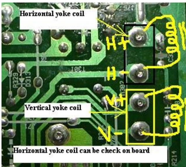
I personally owns an inductance meter and when I compared a known good yoke coil with a bad one, the result was still the same (good inductance value) but when I compared and checked it with dick smith meter, it clearly distinguish between the good and the bad yoke coil.
