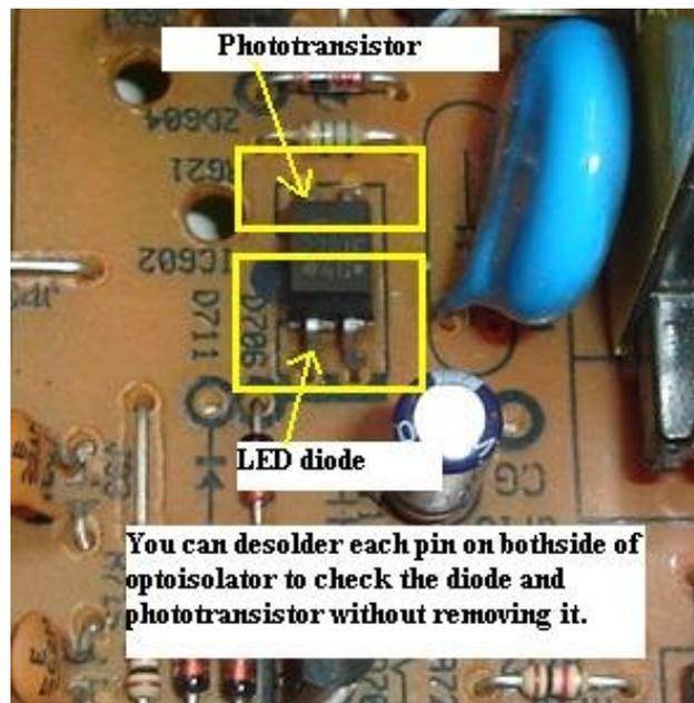
Optoisolator or optocoupler IC's usually located in between the primary and secondary side of power supply and can be test even if the IC is still
