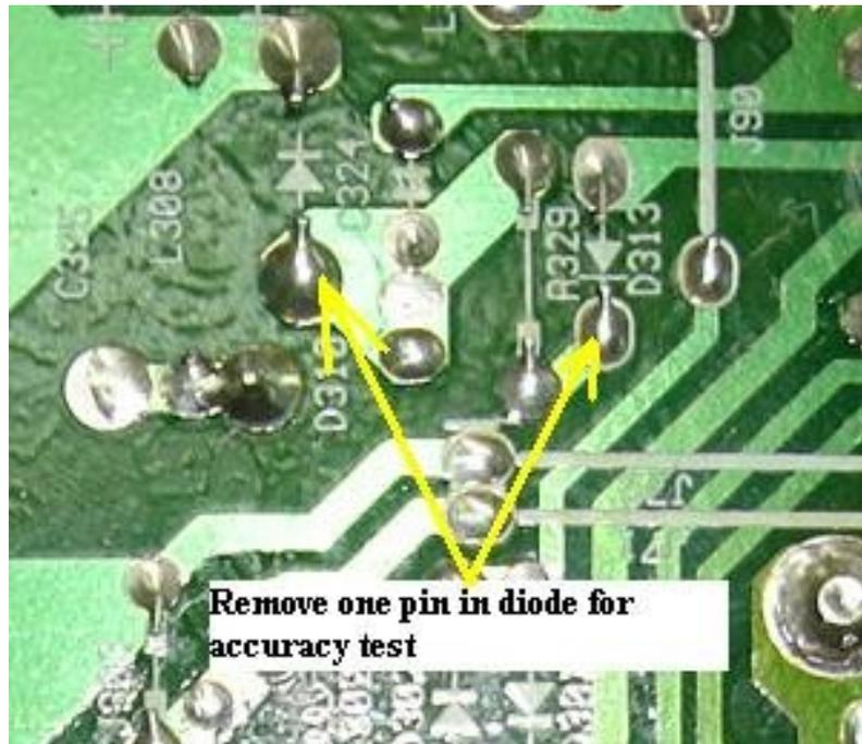
In order to accurately check diodes, you need to desolder one lead and test it with an analog meter set to X 10k ohms range. A good diode should have only one reading while the bad one will have two readings. Be careful if you want to test a Schottky diodes as Schottky diodes will have two readings but not shorted readings. If you get two similar readings then the Schottky diodes is considered bad.
