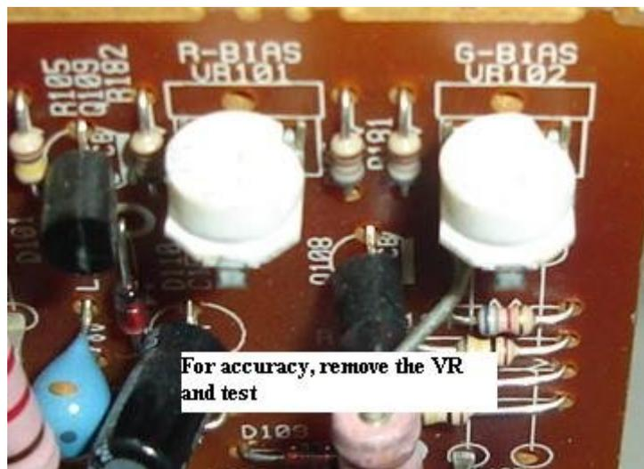
Checking variable resistor (VR) on board is not that accurate because of the back circuit besides some VR have their resistance code printed so small at the bottom of the VR. The best is still removing it out from the circuit and test it with an analogue meter. Any erratic reading can be easily seen from the analogue meter panel compares to using digital meter.
