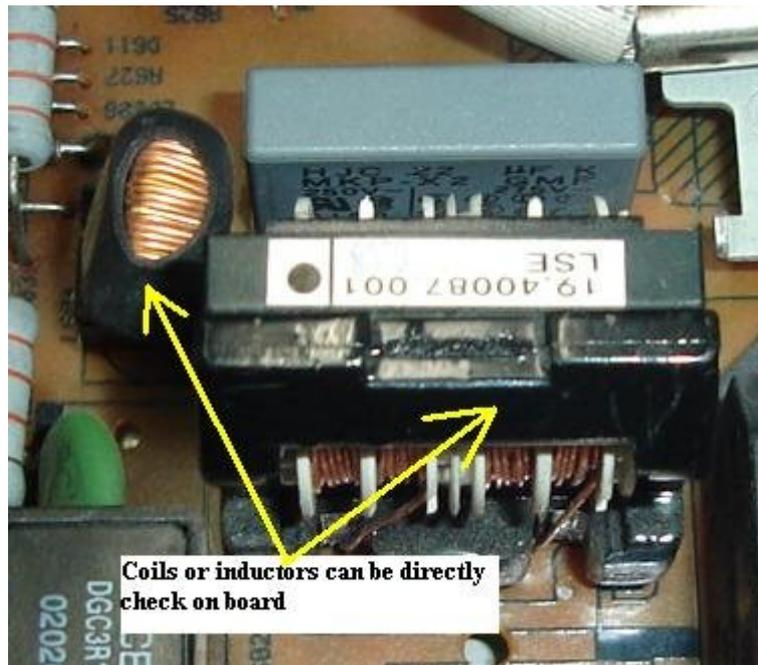
Inductor or coil testing can be done on board without removing the coil out from the circuit board. If a coil has less loops (small coil), then we can just direct measure it with our normal ohmmeter. A small coil is just like a wire or a jumper and it rarely become defective although it has some inductance value in it. Testing coils that have a bigger inductance value like the B+ coil used in Monitor circuit is different from checking the small coils.
