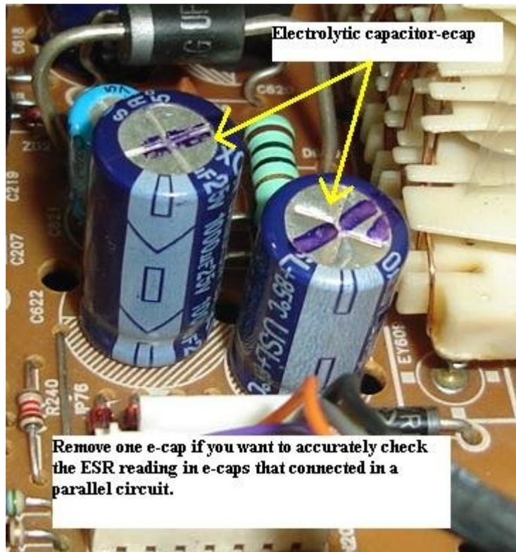
What I mean ESR meter can't test accurately on board in all circuit was that it depends on what type of circuit you are checking! If you check on the Monitor heater circuit, it would not give you an accurate reading because the heater line is eventually go to cold ground through the filament inside the CRT tube. In other words you are actually measuring the low resistance winding of the filament.
