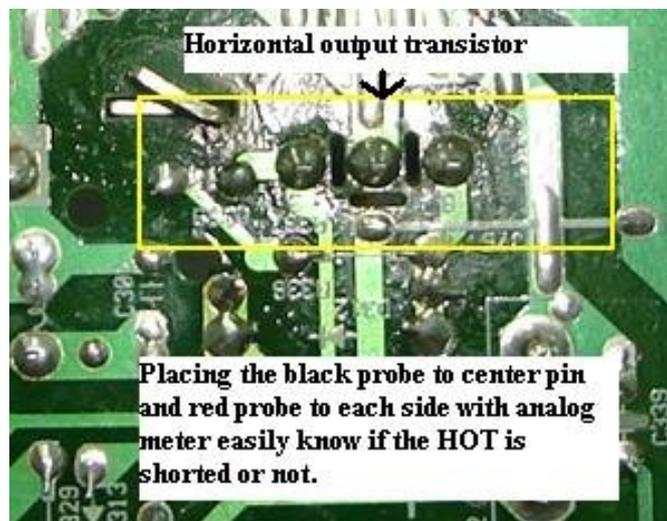
Checking horizontal output transistor is so easy and you can check it on board. Set your analogue meter to X 1 ohm and place the black probe to the centre pin (collector) of the HOT and the red probe to base and emitter. It should not register any reading. If there is a reading, most probably the HOT has developed a short circuit.
