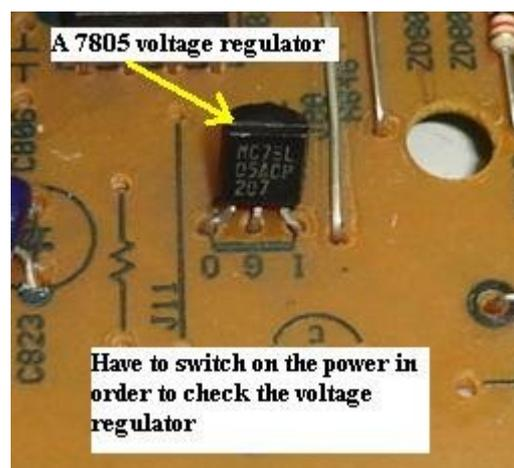
Voltage regulator can't be check off board with multimeter because it is an IC (it has lots of components inside it). You have to switch "ON" the equipment and check the output dc voltage of the voltage regulator. First you must know what the part numbers of the voltage regulator are, and then you read the specification and locate the input and output voltage and pins. For example, the general type of voltage regulator starts with the part numbers like 7805, 7812, 7908 and etc.
