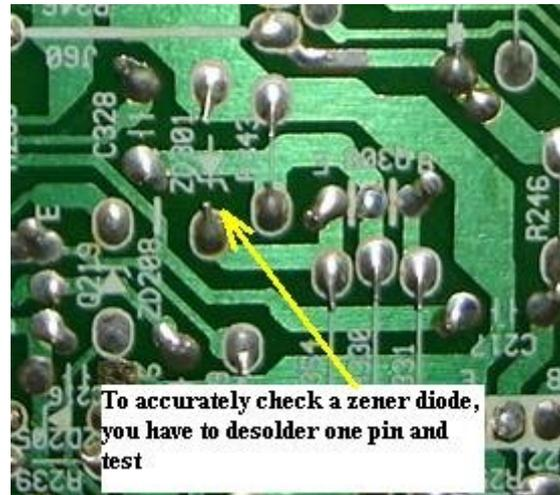
Checking zener diodes, you have to remove one lead from the board. Before you check on any zener diodes, you first need to identify what is the voltage of the zener diodes. Refer to semiconductor data book for any codes printed on the body of zener diodes. Once you know the zener diode voltage, by using again analogue meter set to X 10 K ohm range, you will quickly determine if the zener diode is faulty or not.
