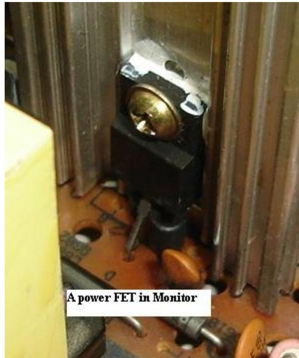
Many switch mode power supply are using the combination of a power FET and a PWM IC design to switch the power transformer. Whenever there is any power failure (fuse totally blown into dark colour) one will always suspect the power FET has gave way. Usually we would use the black probe set to X 1 ohms and place it to the centre pin (drain) and the red probe to the gate and the source pin.
