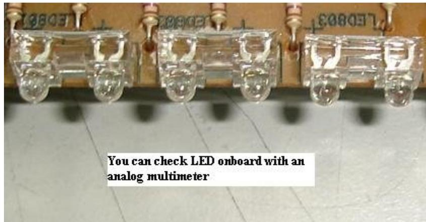
Light emitting diodes or LED is very simple to check. Just connect your analogue meter probe to the pins of LED and set your meter to X1 ohm. If there is no light from the LED, just change the polarity of the probes. You can check LED while it is still in circuit.
