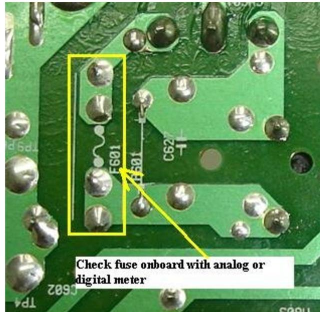
Next is the fuse, you can easily check it on board with your multimeter. Just set your meter either to ohms or continuity. A good fuse should have reading (ohms value) and beep sound if you select the continuity test. If no reading or sound, 100 % the fuse is open and need replacement. Replace only with the same ampere and voltage rating of fuse.
