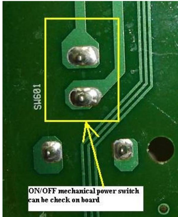
Checking the on/off power switch is the easiest one. Just place your meter probes to the switch point (assuming the power switch have 2 leads) and set your ohm meter or continuity check function. It should show a very low ohm resistance or the beeper will beep if you use the continuity checker. You can perform this test even if the power switch is still in circuit. You can also use this method to test on the micro switch.
