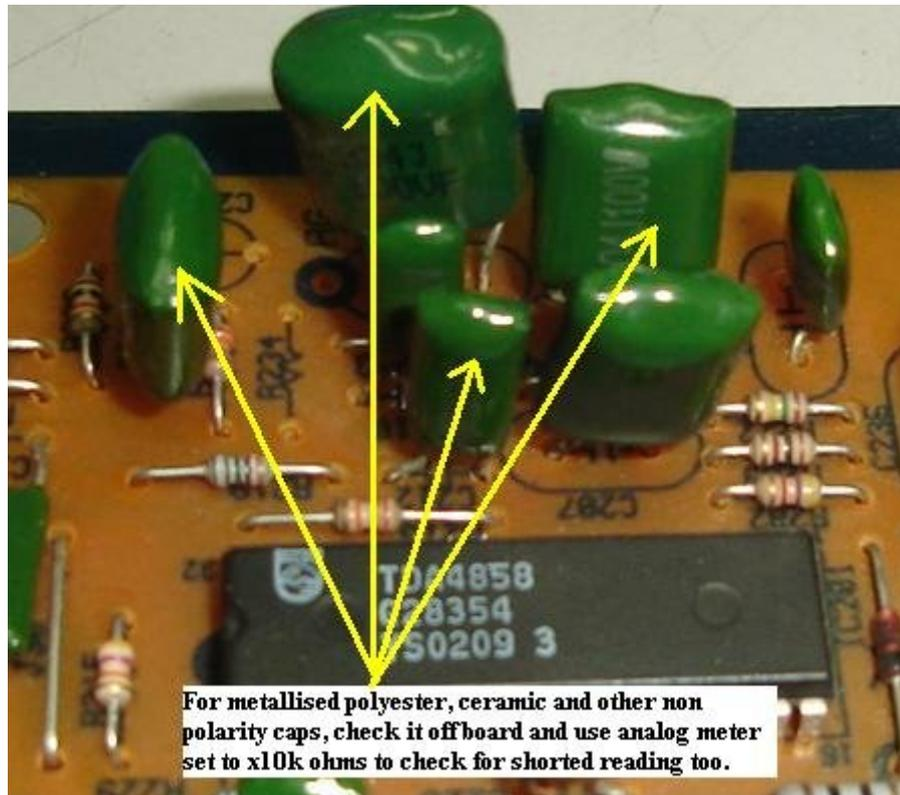
Next is the non polarity capacitor, you have to desolder on lead in order to test the capacitance. You can't measure the non polarity capacitor on board as the digital capacitor meter doesn't have the capability to check on board not like the ESR meter. After you have confirmed that the capacitance is good you need to perform another test which is using analogue meter set to X 10 k ohm to check for any short circuit between the internal plates.
