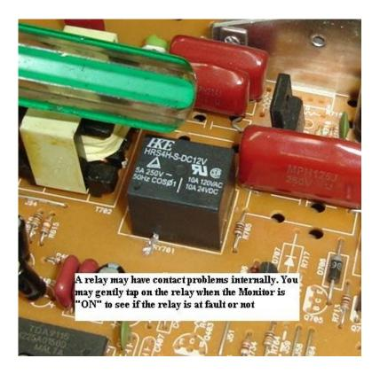
A loose contact inside relays also may develop intermittent problem. Just tap on the relay when the equipment is working to see if there are any changes. Be careful when you are tapping the relay as the power is on. Replace with a new relay if you suspect it is the cause of the intermittent
