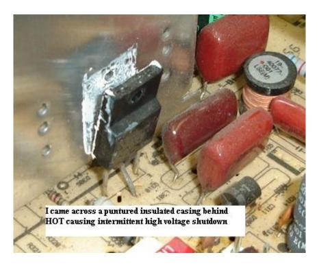
Intermittent problems can be tough to work on if you do not know the necessary steps to tackle it. Absorb all information in this article to localize the problem because it is far easier to check and test a few things than to check every joint, contact, and component in the equipment. Have a great hunt my friend!
