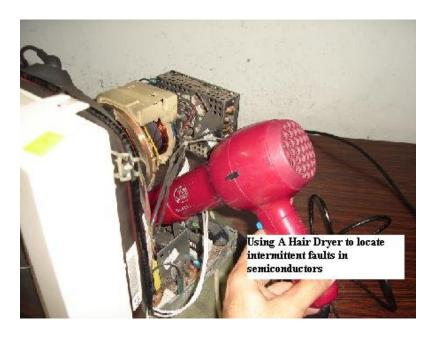
Next is the thermal intermittent problem, where a component works okay when it is cool and problem arises when in the high temperature. In order to detect such problem, we need to use a little heat so that the problem can surface faster without you wasting hours to wait for it to happen. By placing a 100 watt bulb near the board of the equipment, the circuits will become quite warm after a few minutes. You may also use a hair dryer to point or focus on the circuit board.
