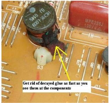
There was one case where the Monitor was switch "on", it has intermittent shutdown problem. I really spent lots of time trying to tackle the faults from behind the board. Flyback transformer replaced, PC tube changed, voltage testing on all circuits to be okay, but somehow I just could not locate the cause of the problem.
