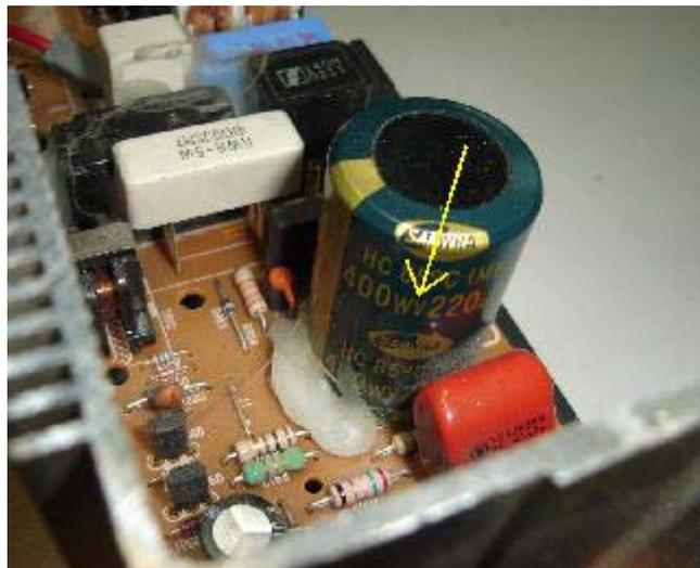
A Filter Capacitor in Switch Mode Power Supply
