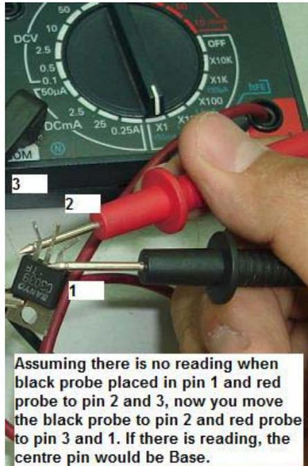
The diagram in Figure 2 assumes you are testing an unknown type of transistor. Set your meter to the lowest ohm's range i.e. **Rx1Ω**. From the six combination of test result you will know the transistor is belonging to which type.
