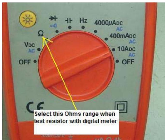
Personally I do not use analogue meter to test resistor as the result shown on the meter panel only makes you have to guess what the resistor value is. You may ask yourself, is it 47 ohm or 47.5 ohm or even 47.7 ohm? By using digital meter the LCD display in your meter will show you the exact value of the resistance under test. It is more accurate than using analogue meter.
