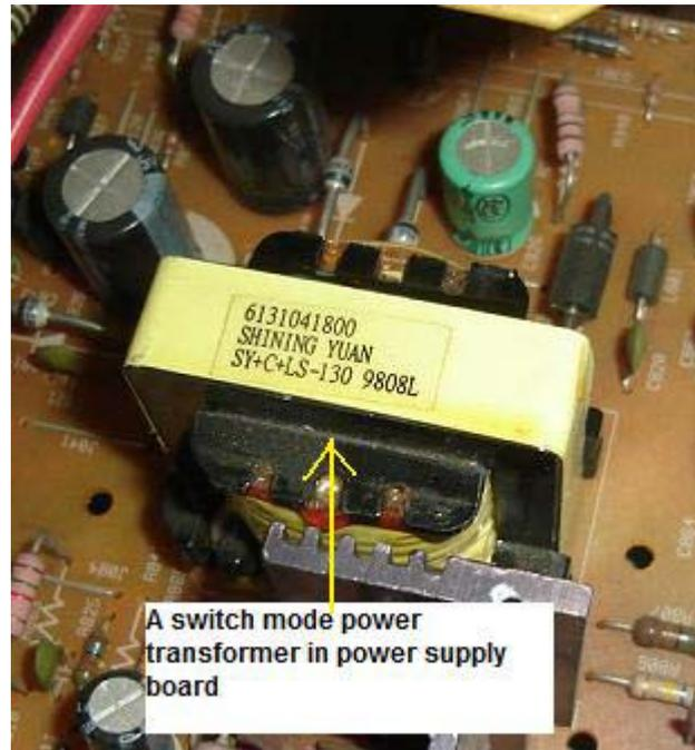
A switch mode power transformer in power supply board
