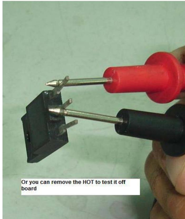
Conclusion- If you measure base (black probe) and collector (red probe) it should have reading.
