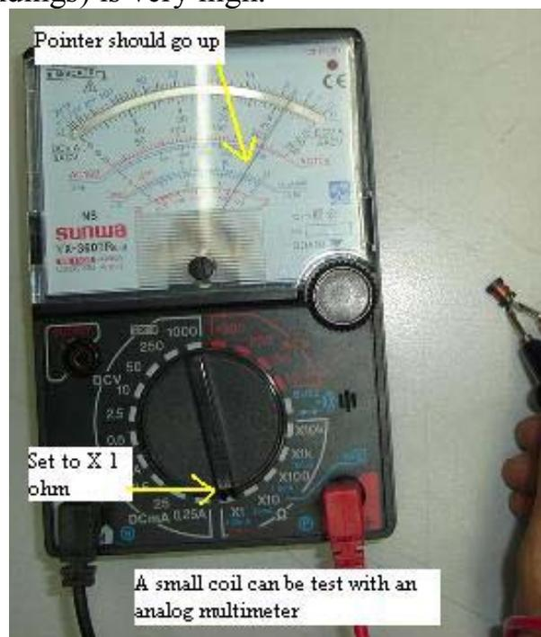
Testing bigger coil or inductor such as the computer monitor B+ coil, you need an inductance meter to find out the exact inductance value which is in the unit of Henry (h). From experienced using an inductance meter to check coils to see if it good or bad is not recommended because a shorted coil (shorted between winding) could have a good inductance value and you would miss out checking a bad coil.
