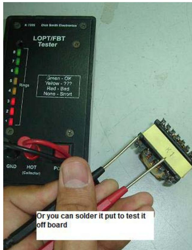
Placing the flyback tester probes to the primary winding of the switch mode power transformers, a good measurement will usually be between of
