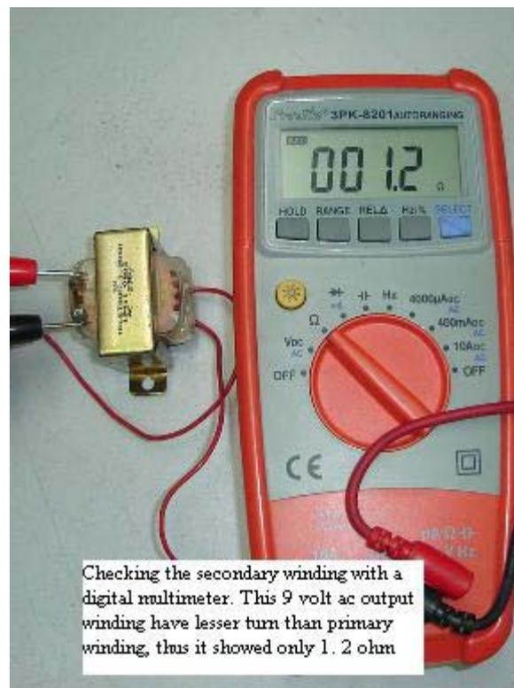
Checking the secondary winding with a digital multimeter. This 9 volt ac output winding have lesser turn than primary winding, thus it showed only 1.2 ohm
