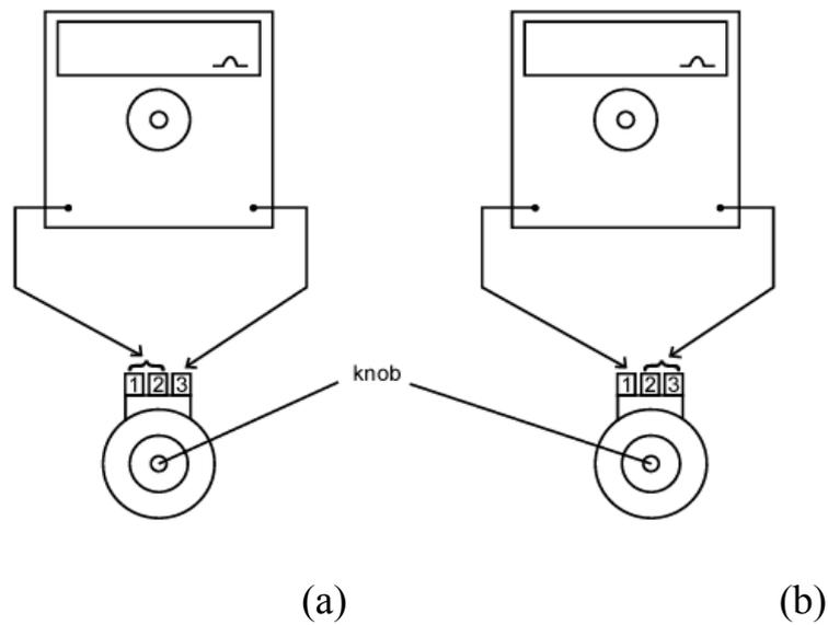
Fig 1: Testing a variable resistor with a analogue multimeter
