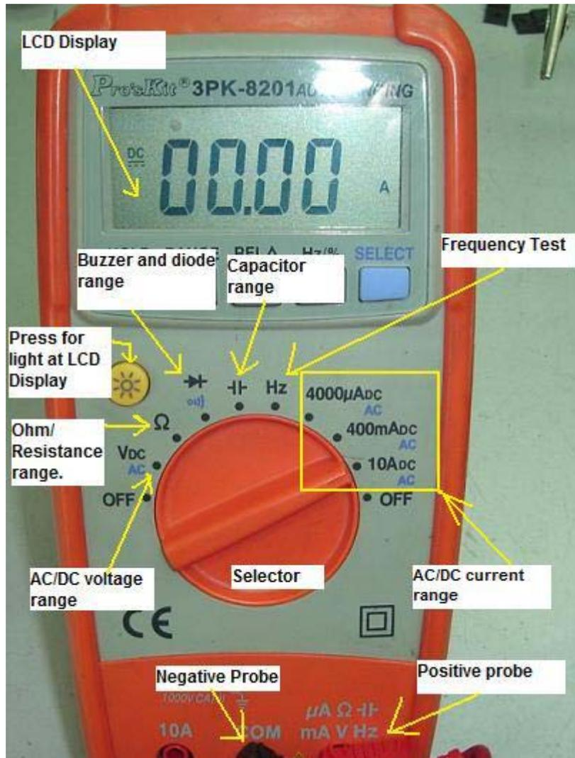
Black test lead plugs into meter terminal marked Common, Com, or  $\ominus$
