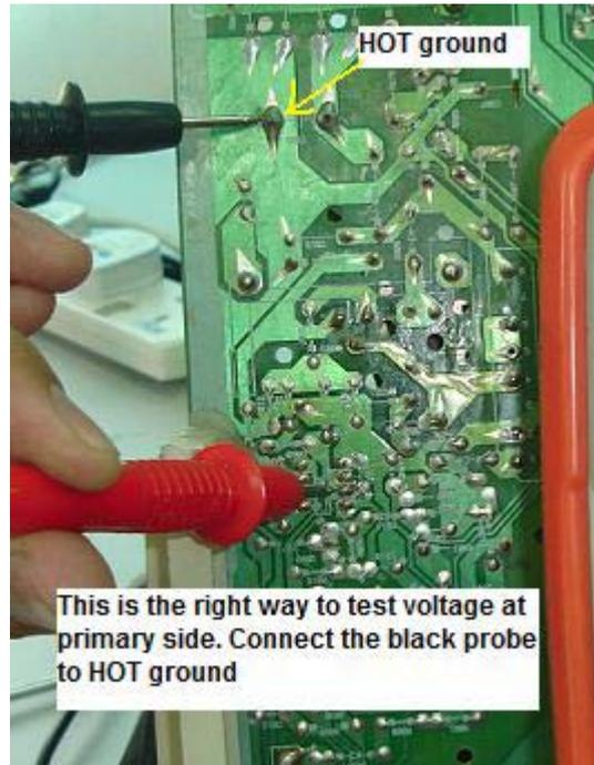
**Warning: A switch mode power supply has primary and secondary section. In order to check secondary voltage the meter's black probe have to connect to cold ground (chassis ground) and if you want to test on the primary voltage, the black probe have to connect to primary ground! If you are not familiar of what I am saying, please ignore this test or get a repair friend to assist you.**
