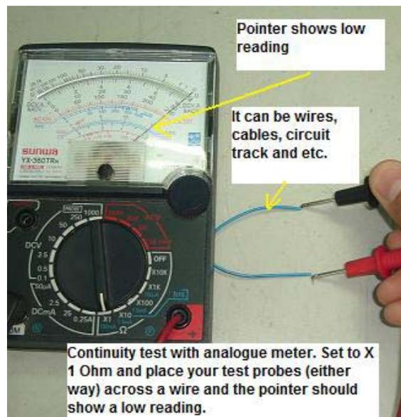
Now, connect the two probes to the points where the short or continuity is to be checked as shown in the photo in previous page. If the meter shows zero Ohm, it means the continuity is present or the connection internally not broken. Ideally, a good continuity should be about 0 Ohm.
