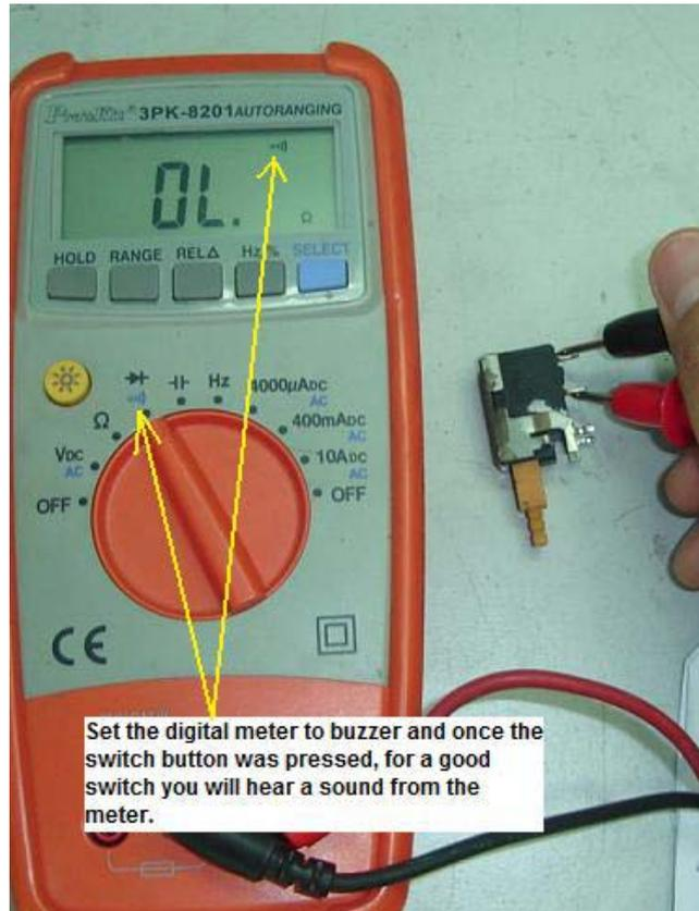
If after pressing the switch and nothing happens, suspect a bad switch. Similarly, you can use a digital meter set to buzzer sound to test a switch. A good switch with a good contact should make the digital meter to produce the buzzer sound. No sound means the switch is defective.
