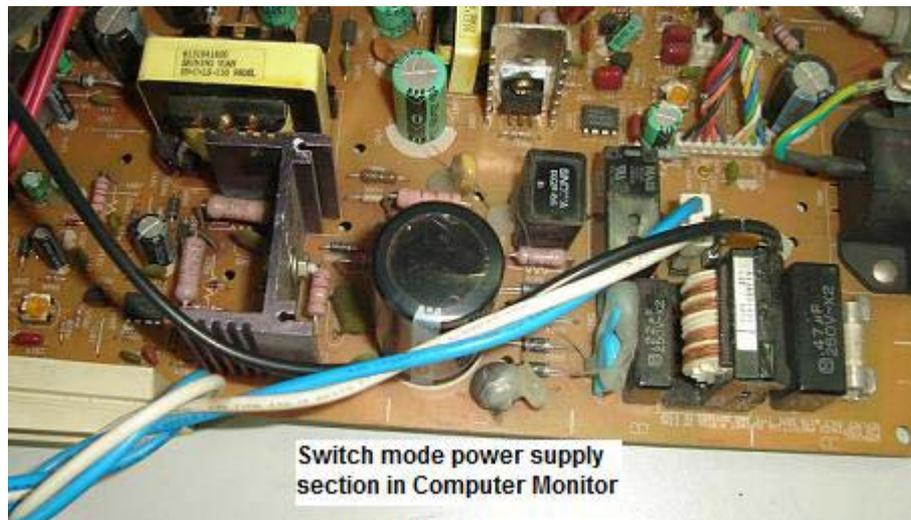
Switch mode power supply section in Computer Monitor
