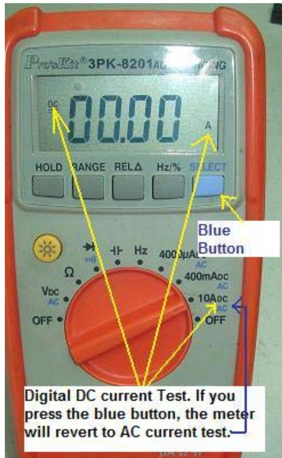
Inserting a meter in series, however, is not always an easy task. In many cases you must physically interrupt a circuit at the point you wish to measure, and then connect test leads across the break. Although it may be easy to interrupt a circuit, keep in mind that you must also put the circuit back together.
