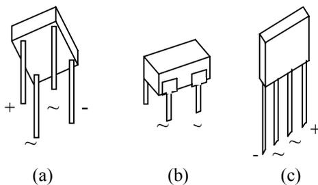
Fig 1: Some examples of bridge rectifier
