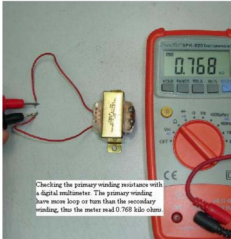
Checking the primary winding resistance with a digital multimeter. The primary winding have more loop or turn than the secondary winding, thus the meter read 0.768 kilo ohms.
