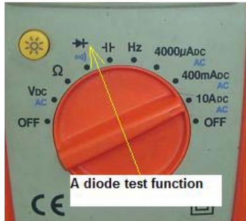
If you don't get any reading either forward or reverse bias, the diode is considered open circuit. The real problem when testing a diode using the diode test function of a digital meter is that an open or leaky diode, the meter sometimes reads okay. This is due to the digital meter diode test output voltage (which you can measure the output test probe using another meter) is around 500mv to 2v.
