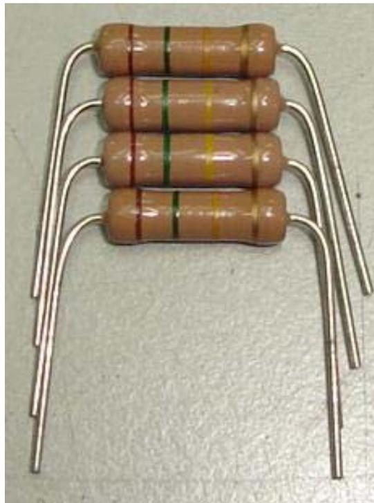
The main two characteristic of resistor are its resistance R in ohms and its power rating in watts, W. Resistors are available in a very wide range of R values from a fraction of an ohm to many mega ohms. The power rating may be as high as several hundred watts or as low as 1/8 watt. Always use a replacement resistor with a power rating that is equal to or greater than the original. The value of the resistance can be measure by a multimeter.
