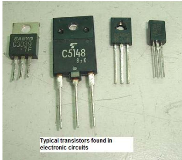
Transistors are solid –state devices similar in some way to the diodes you have studied. Transistors are more complex and can be used in many more ways. They are very important and can be found in almost all modern electronic equipment. The name transistor is derived from “trans resistor”, meaning that it **changes resistance**. Unlike a diode, a transistor has three leads. The three transistor leads are designated as **Base (B), Collector (C), and Emitter (E)**.
