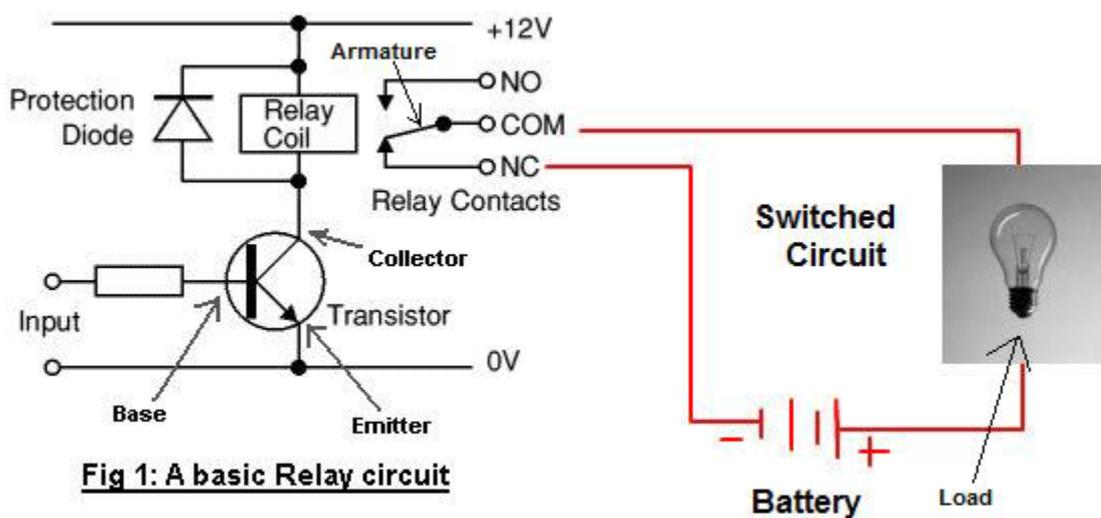
Figure 1 show a basic relay circuit. If there is an input signal going to the base of transistor, the transistor will conduct and the 12V will flow through the relay coil, the collector, out from emitter and to ground (0V). This will energize the relay coil and cause the armature to switch from the “normally close (NC)” to “normally open (NO)”. When the armature in the “normally open (NO)” state, no current will flow to the lamp (load) and the lamp will go off.
