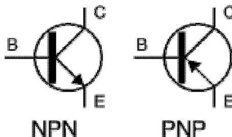
Fig 1 : The circuit symbols for the two transistor types a) NPN b) PNP
