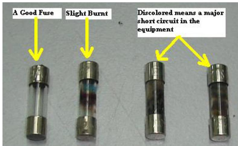
A blown fuse can indicate how severe the short circuit is.
