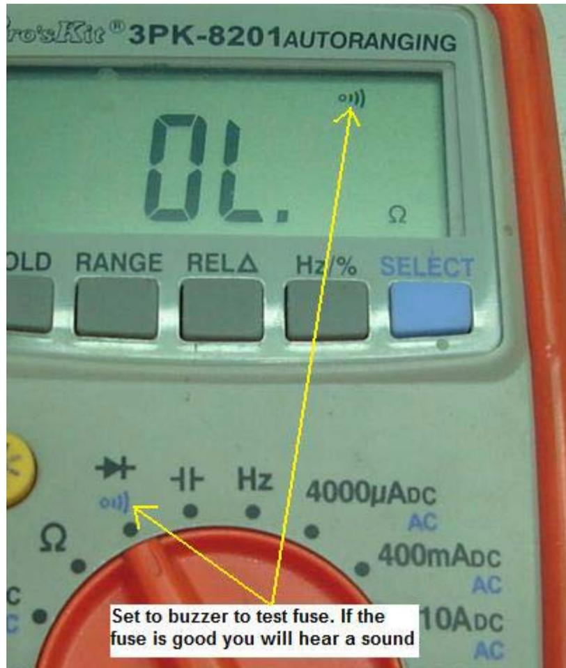
Setting buzzer range to test a fuse with digital meter
