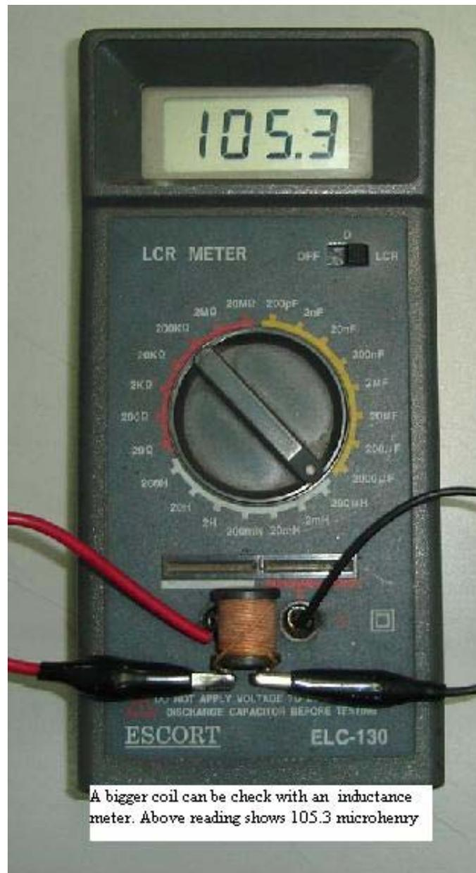
A bigger coil can be check with an inductance meter. Above reading shows 105.3 microhenry
