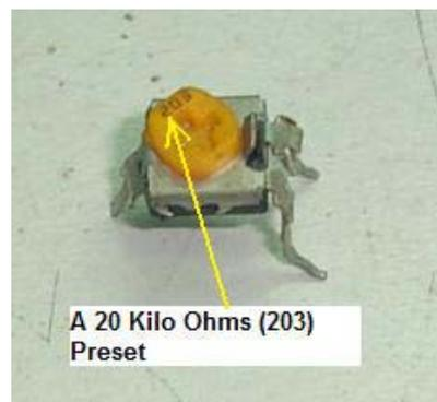
These are miniature versions of the standard variable resistor. They are designed to be mounted directly onto the circuit board and tuned only when the circuit is built. For example to set the colours of Computer Monitor by turning the preset in the Cathode Ray Tube (CRT) board.
