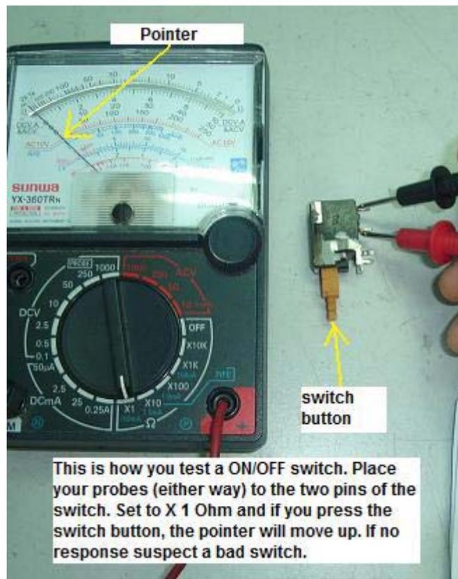
This is how you test a ON/OFF switch. Place your probes (either way) to the two pins of the switch. Set to X 1 Ohm and if you press the switch button, the pointer will move up. If no response suspect a bad switch.
