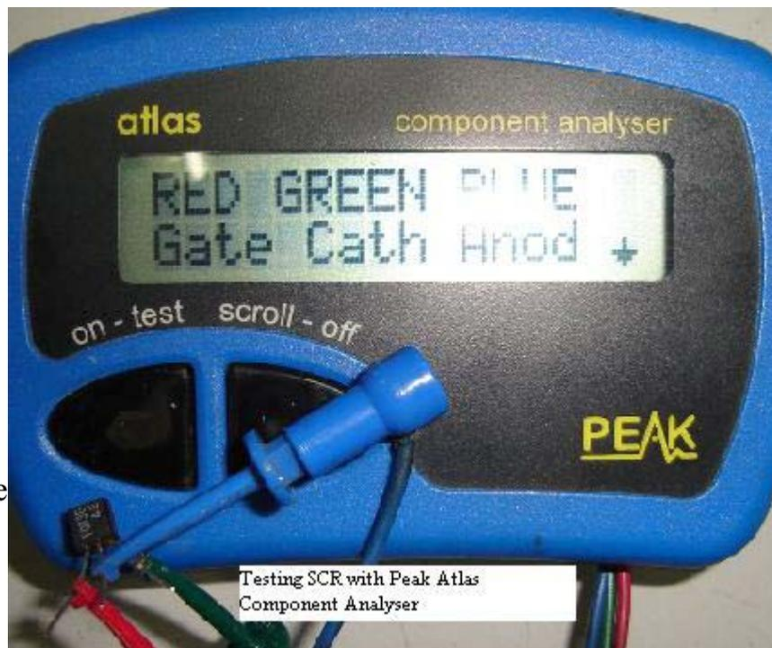
The tester will begin to analyze the SCR and prompt you with the display such as “Sensitive or low power thyristor” before it tells you the exact pin outs of G, A and C. After the first test, the tester will eventually show you
