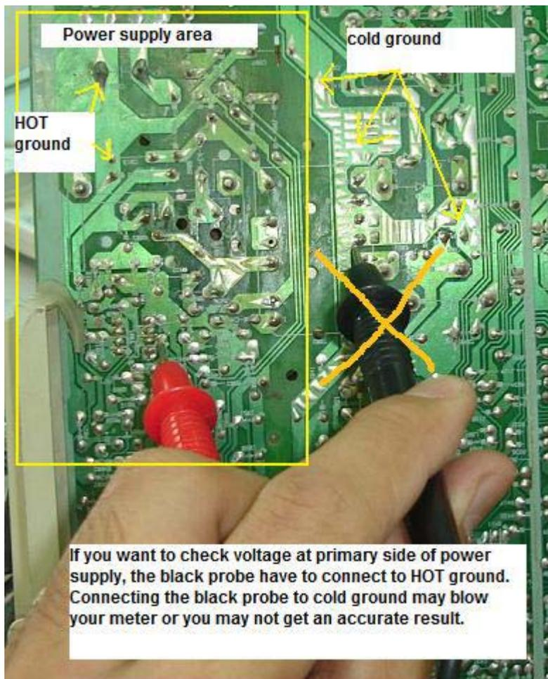
If you want to check voltage at primary side of power supply, the black probe have to connect to HOT ground. Connecting the black probe to cold ground may blow your meter or you may not get an accurate result.
