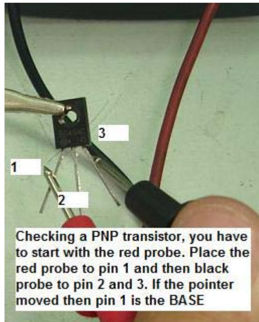
Your test probe placement must be reversed in order to check for PNP type of transistor as shown in Figure 3.
