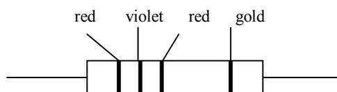
The first band is red for 2 and the next band is violet for 7. The red multiplier in the third band means add two zeroes to 27. The result can be illustrated as follows:
