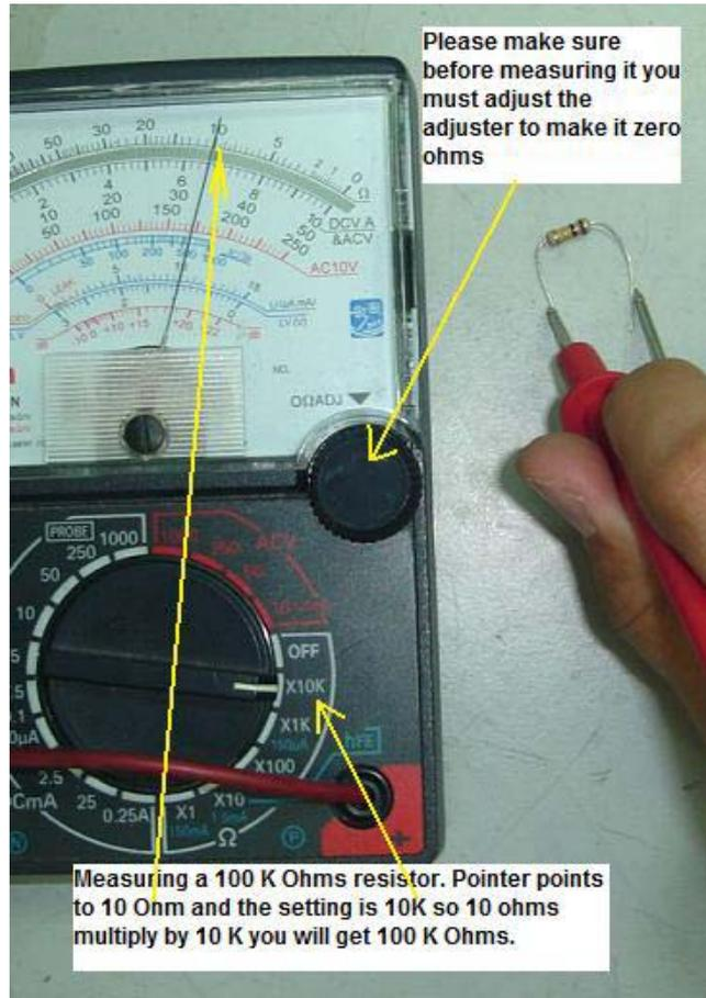
In order to check a 100 K ohm resistor you have to select the X 10 K Ohm range. Follow the procedure explained above and you should be able to get the measurement.
