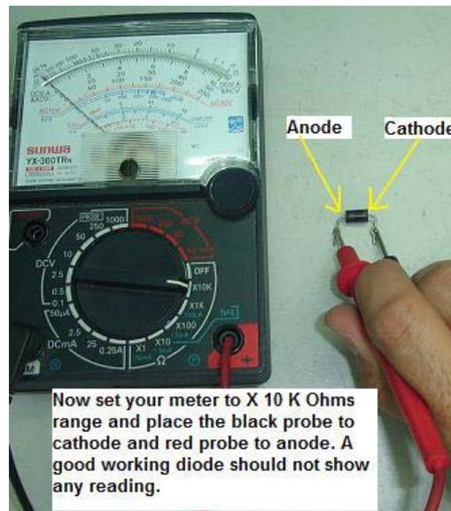
You now have to select your meter to x10Kohm range to test the diode again. The output voltage of x10k ohms is about 12 Volt (remember the 9 volt battery in your meter-1.5 volt + 1.5 volt + 9 volt = 12 volt). Again the diode under test should show only one reading. This is exception to Schottky diode where it has two readings but not shorted reading. I will explain how to test Schottky diode in the next section.
