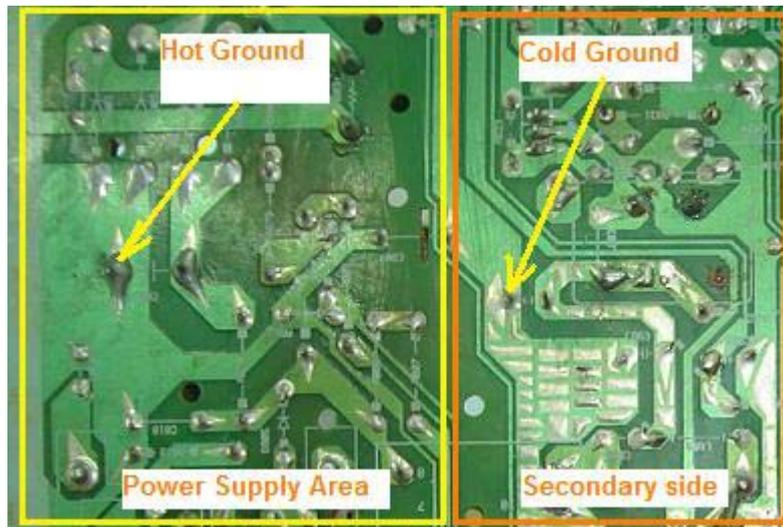
Modern equipment consists of two grounds, one of which is a “hot” ground while the other is a “cold” ground. Hot ground is in the primary side of a switch mode power supply while the cold ground is the equipment ground.
