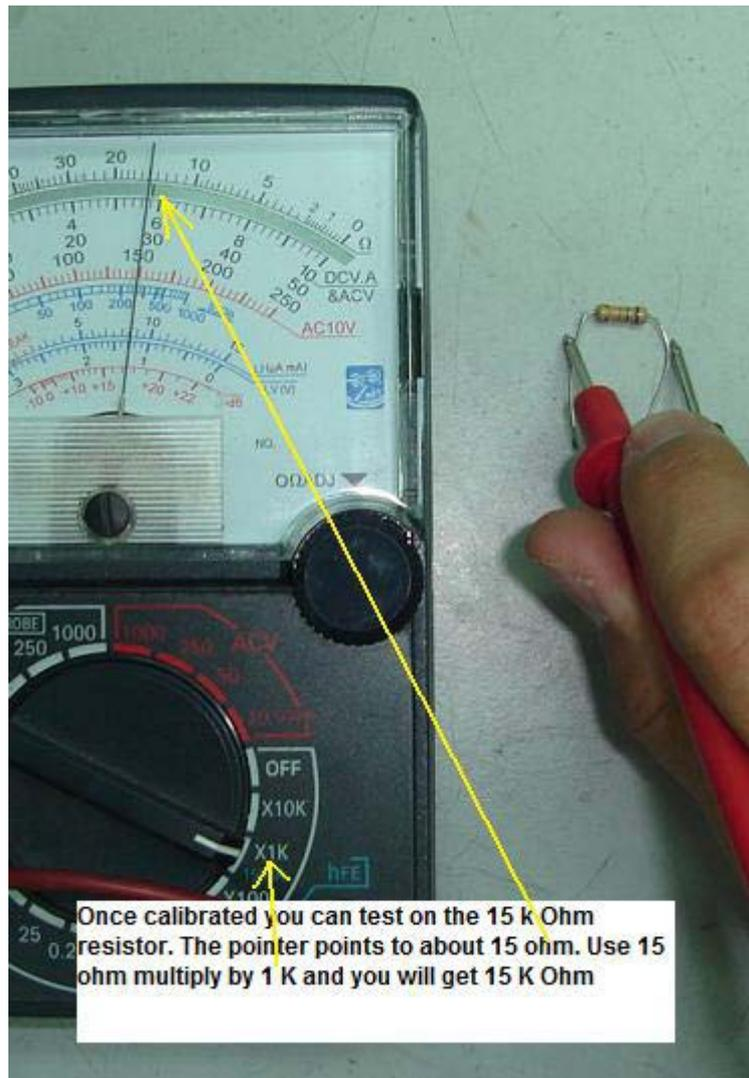
Check the result to see if the pointer point to near or exact 15 K Ohm. If the resistor has 5% tolerance the pointer should point between the values of 14.25K to 15.75K Ohm. Any value you get that is not between the tolerance ranges, you should replace the resistor.
