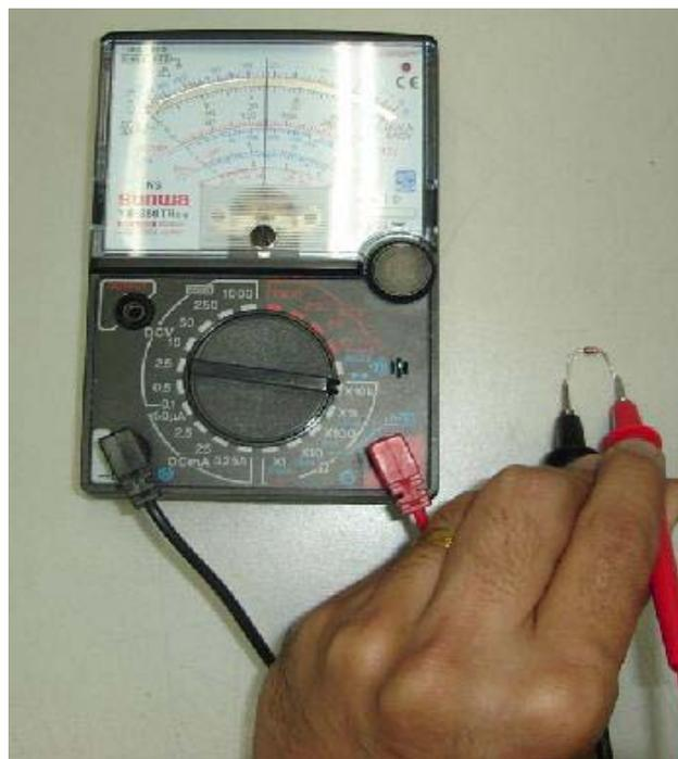
Use analogue multimeter to test zener diode
