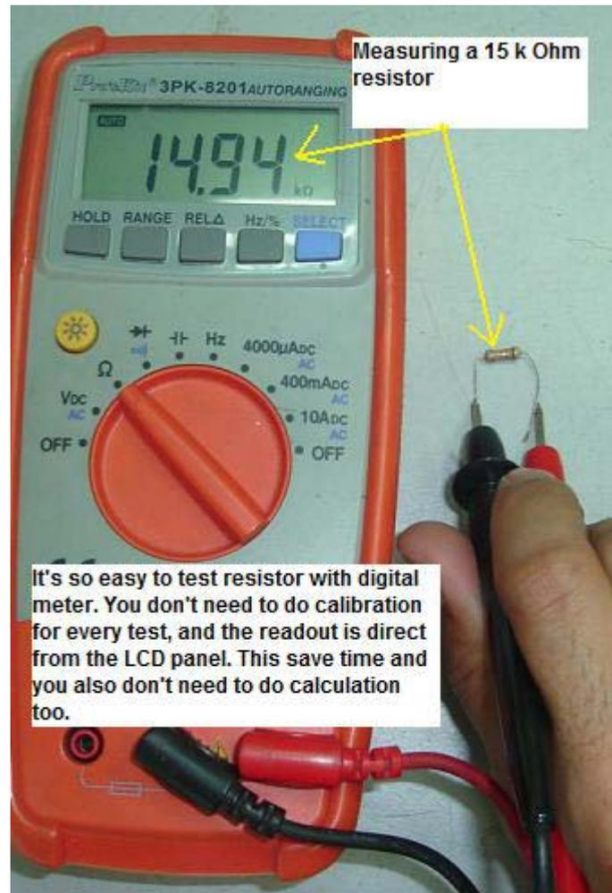
First, select the Ohm range and place your test probes across the two points of the resistor as shown in the photo. **Digital meter does not need any calibration compare to analogue meter** where you have to adjust the adjuster to make it zero Ohm before you begin to do measurement. The result shown at the LCD display of the digital meter is the exact resistance value of the resistor.
