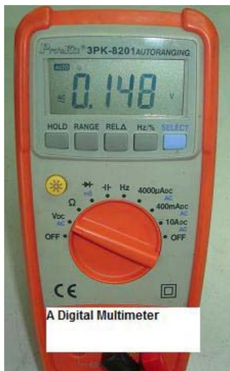
Multimeters (analogue and digital) are one way in which you can “see” what’s going on in an electrical circuit. Voltmeters, ohmmeters, and ammeter are essential in all electric work. Multimeters can go by many
