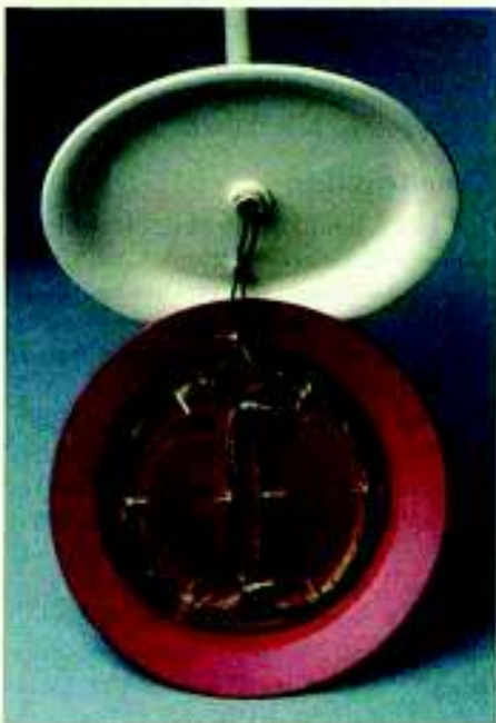
This photo clearly shows the potted search coils in situ.
