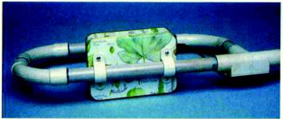
This photo gives you a better idea of how the electronics box is mounted to the main PVC pipe. Ordinary saddle clamps hold it in place.
