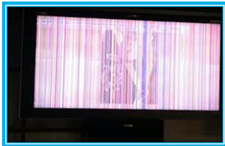
Philips T-Con Failed
