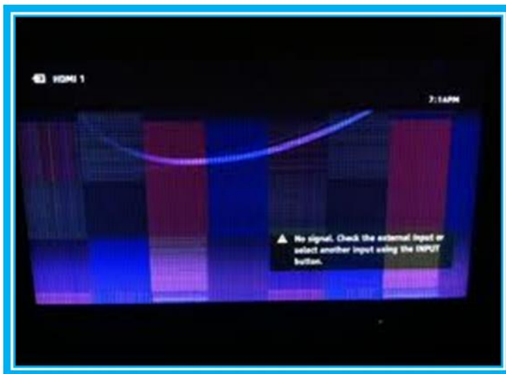
Samsung T-Con Failed
