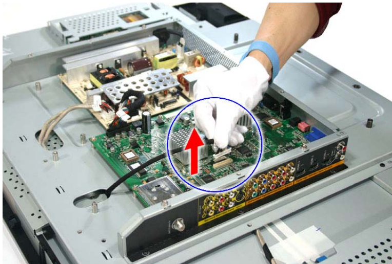
LVDS cable, requires screw removal (above)
