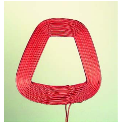
Figure 3. The author's original pick-up coil.
